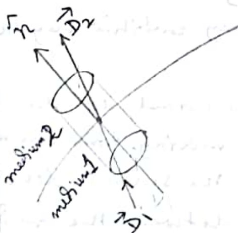
fig.1: Boundary condition on the normal comp. of \vec{D}
